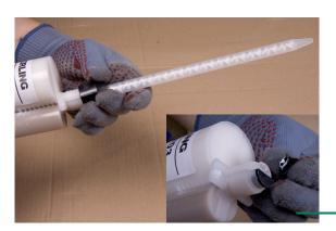
Open Tandem Cartridge, attach Static Mixer and screw it tightly with locking cap;
