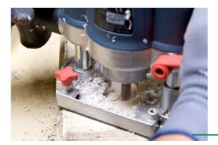
**4.** Position Router above damage and mill off the damaged area.
