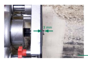
**3.** Choose a Milling Head, depending on damage size, and adjust it to approx. 3 mm depth.
