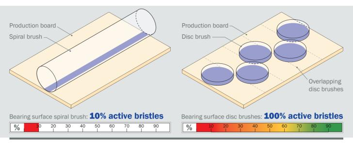
Spiral brush and Crust Cracker<sup>®</sup> in comparison
