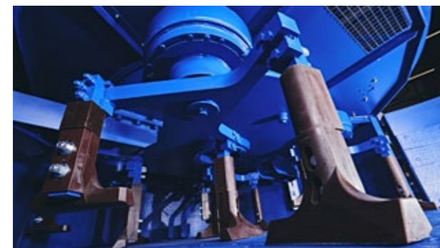
Robust mixing tools with wear protection ensure a long service life and optimum mixing results in the main concrete mixer.
