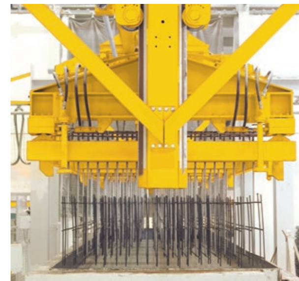
Placement of reinforcement elements
