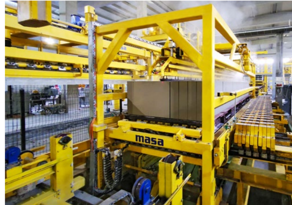
Green separating table with product-related adjustment of the separating beams
